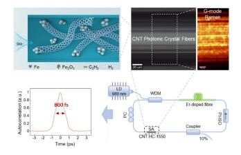
Direct growth of carbon nanotubes (CNTs) with narrow diametre distribution on the inner walls of photonic crystal fibres by a two-step chemical vapour deposition method was developed. By using the as-fabricated 3-cm-long CNT-fibres with desirable nanotube optical transitions, both third-harmonic generation has been largely enhanced and mode-locked ultrafast laser has been fabricated with a stable output of ~10 mW, ~800 fs pulse width and ~71 MHz repetition rate.
